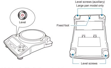
Level the balance by following the procedure below.
