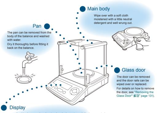
Avoid using organic solvents, chemical agents or cloths impregnated with chemicals since they will damage the coating of the balance and the display panel.
