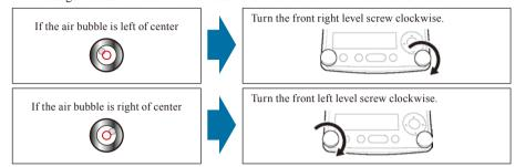
Turn both the level screws at the front in the same direction at the same time to center the air bubble in the level in the front/back direction.
