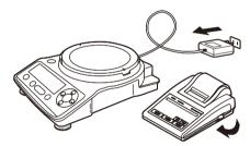
Using the cable supplied as an accessory with the printer, securely connect the DATA I/O connector at the balance and the connector at the printer.
