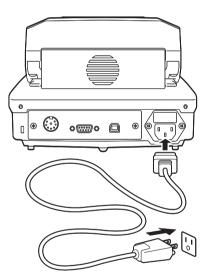
When the power switch is turned on, the version number (\*1) is displayed and the internal system is checked automatically.
