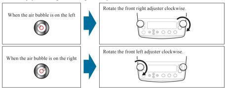
Rotate the right and left adjusters at the same time until the air bubble in the level gauge appears at the longitudinal center.
