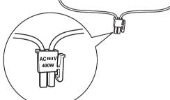
1 Install the heater using the clips.
