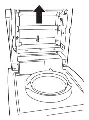
Place the glass case on a flat surface and clean it carefully.
