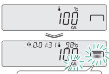
Flashing indicates that heating has begun.
